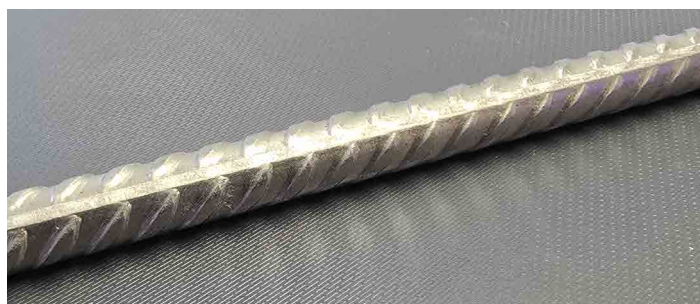
(Figure 2). Example of ribbed cold rolled wire
